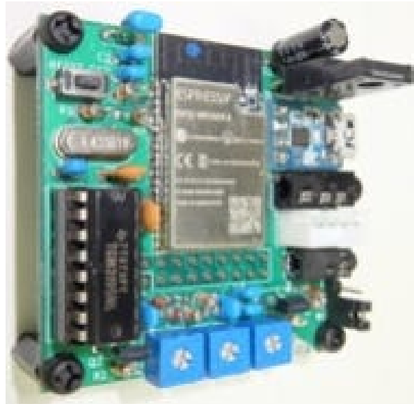
Early version of the PRUG FX.25 TNC, using a TCM3105 modem chip. Image courtesy of Packet Radio User's Group
